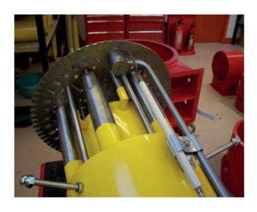
Limpsfield took on the task and designed a twin inlet gas head to accommodate the different flame pattern and velocities of the two gaseous fuels, which allow for easy and quick fuel change over without any hardware changes
