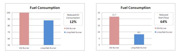
Since the installation of the Limpsfield Burner, Moss have reported a reduction in oil consumption of 12% when compared to the old burner. When coupled with a previous fuel usage of around 200 kg/hr, this translates to significant savings for the client.
